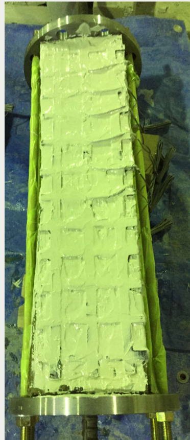
2. Apply the epoxy putty
