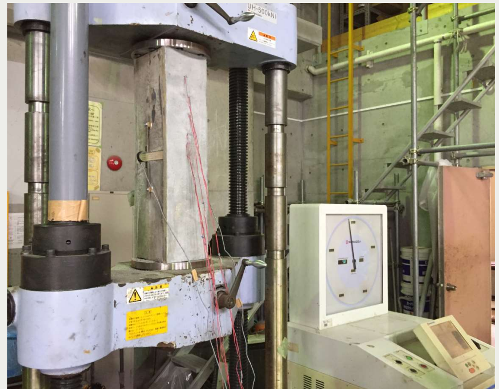
Test setup of double shear test.
