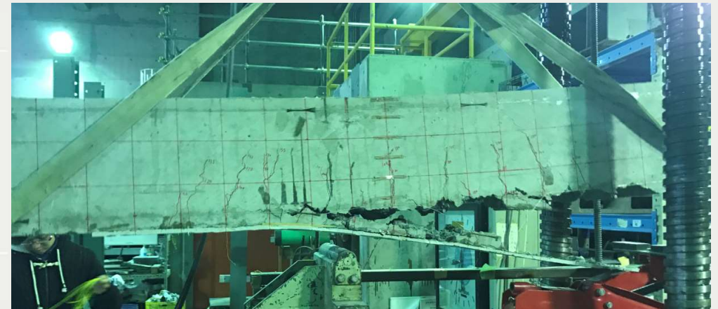
Failure mode of beam [BG-M-PUTTY-5].
