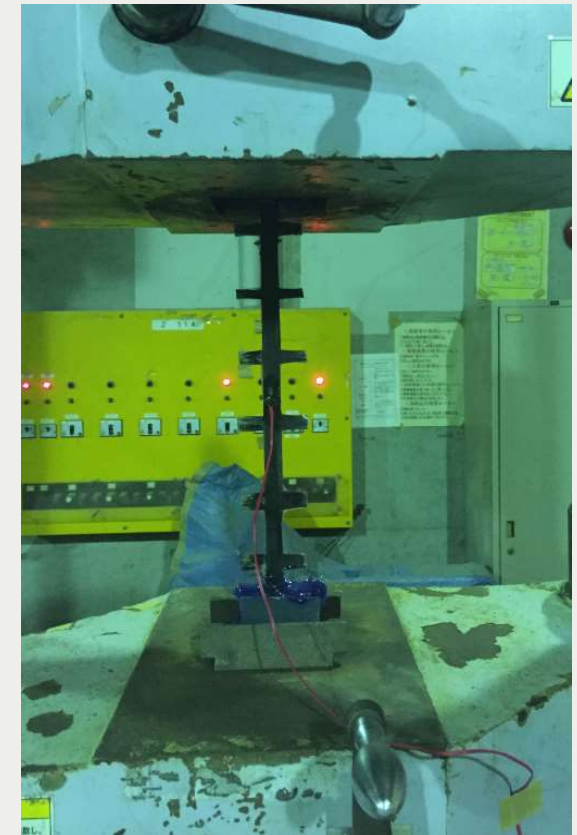
Test setup of BFRP grid.
