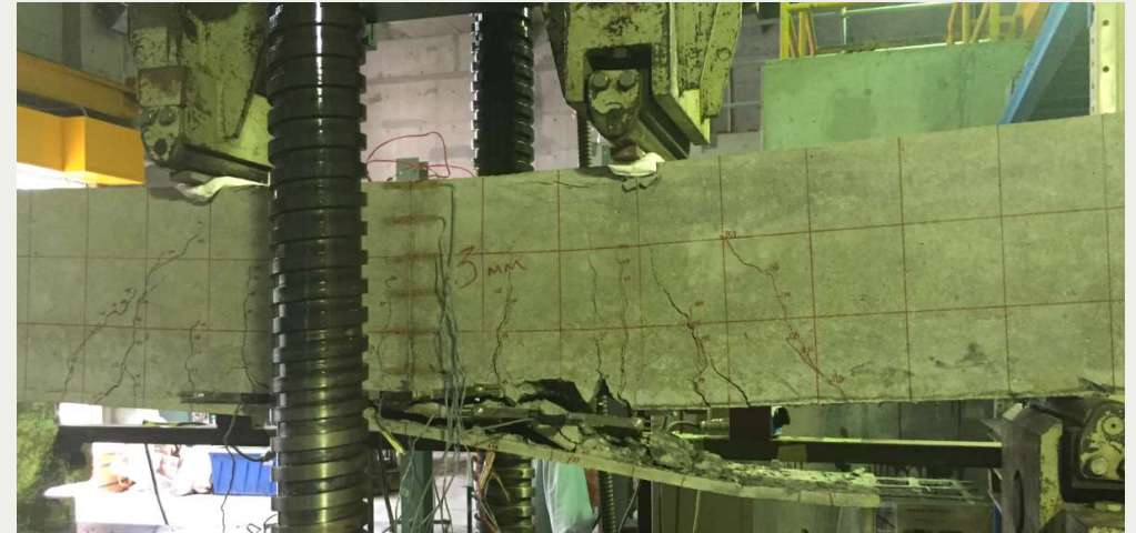
Failure mode of beam [BG-L-PCM-15].
