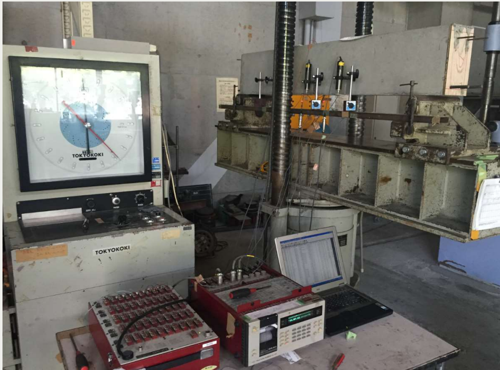
Setup of bending tests of RC beams.
