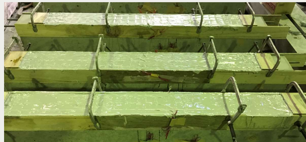
2. Apply the epoxy putty
