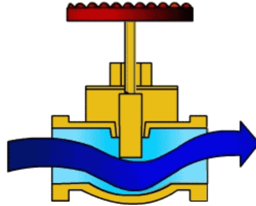
Gate Valve Opened
